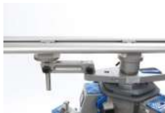
Picture 38 Feeding in of the track end pieces! Sufficiently open the slot nut screws.
