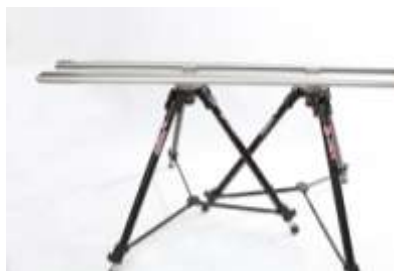
Picture 09 Tracks must be horizontally levelled.
