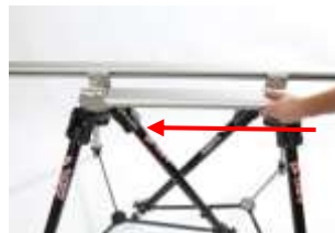
Picture 08 Position the track profile and tighten the slot nut screws with an Allen key.
