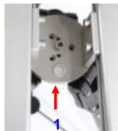
Picture 09 Tracks must be horizontally levelled.
