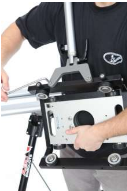
Picture 41 Assembly of the push rod on the dolly frame Use for this the assembly screws (scope of supply push rod)
