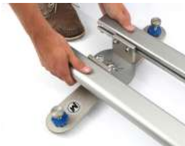
Picture 20 Set the track profiles parallel
