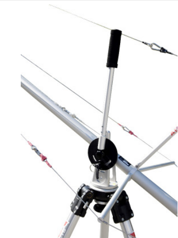
Disc with lever to adjust camera tilt
