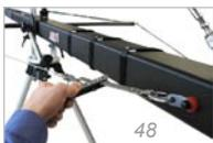
**Fig. 48. Closing the turnbuckle of the outrigger-ropes**
