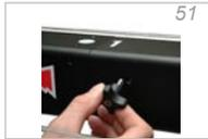
**Fig. 51. Assembly of the segment connecting bolts**
