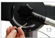
This particularly serves the stabilization in the horizontal position of the crane head when using remote heads. With this adjustment you can always hold the camera in a horizontal position while swivelling vertical.
