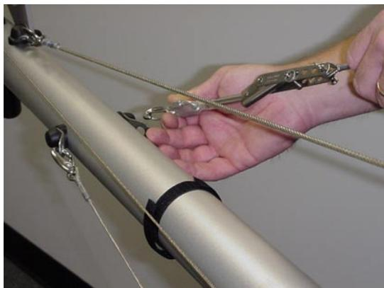
Right hand cable with green mark and tightening clamp is connected at the ring on the right side of the main tube.
