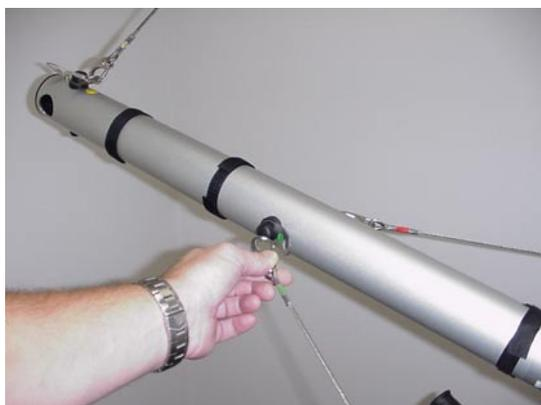
Connect the outrigger cables at the end of the main tube (back end of crane) in a similar fashion.
