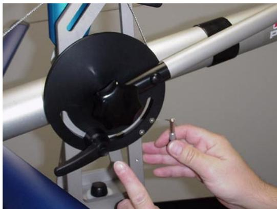
If the camera is tilting up to far, you can loosen the locking lever and with help of the tilt lever, you can correct the camera angle to the desired position. After optimal camera position is reached, the locking lever need to be tightened. The Quick Pin is not used in this set up.
